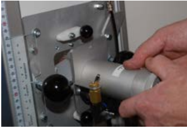
Insert knife head in carriage plate.
