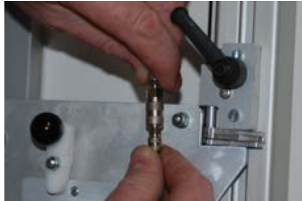
Use airconnector to connect knifehead.
