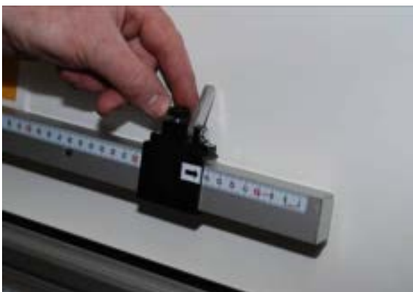
Install measuring stop sizer
