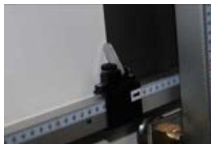
Align matboard to the measuring stop
