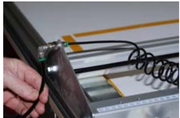
Connect 6 mm air tube on top
