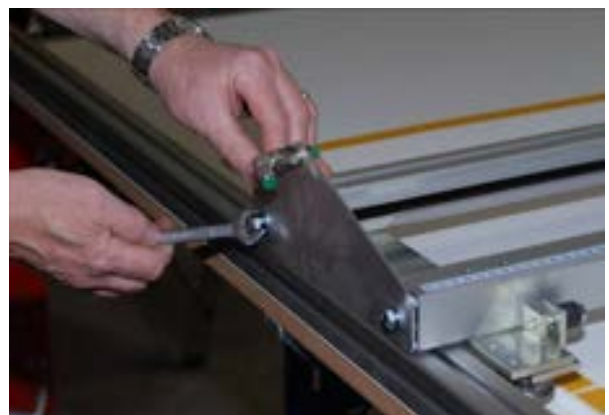
Install connection pneumatic knifehead
