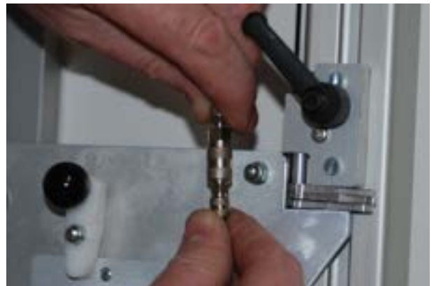
Use airconnector to connect air to knifehead
