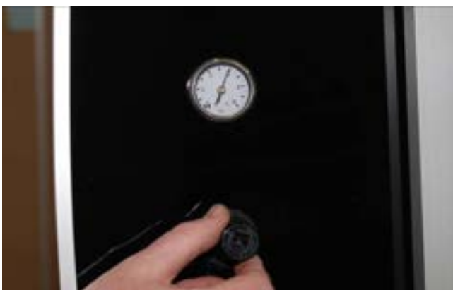
Set pressure knifehead on 6 bar with manual /pneumatic knifehead ,or pneumatic autorotate 3 bar.
