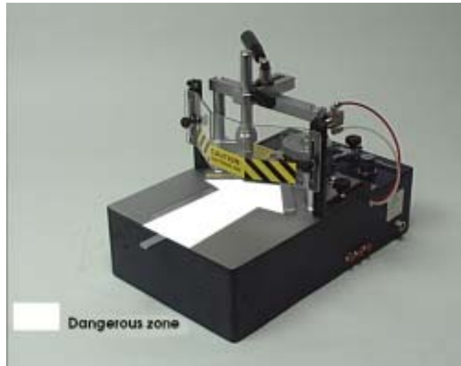
Figure 3.4.A- Working area and dangerous zones
